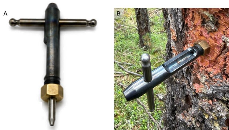
Figure 1. (A) The MoMiC microcorer showing its compact design, transverse handle, and interchangeable sampling point. (B) MoMiC in use for extracting a wood microcore from the stem of a living tree.
